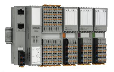
Phoenix Contact AXL F BK fieldbus coupler with I/O
